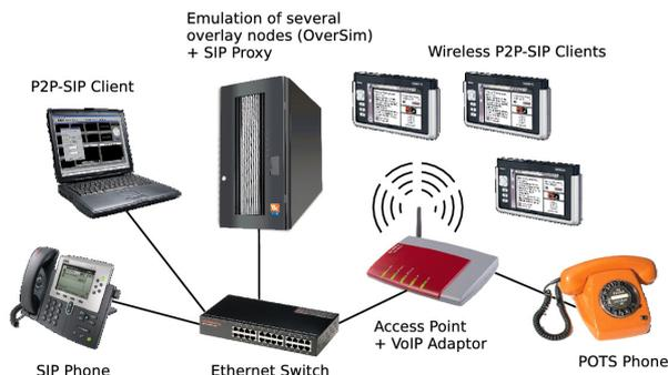
**Figure 6. Architecture of the P2PSIP demonstrator**
